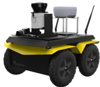
Mobilní robot, UGV - unmanned ground vehicle
