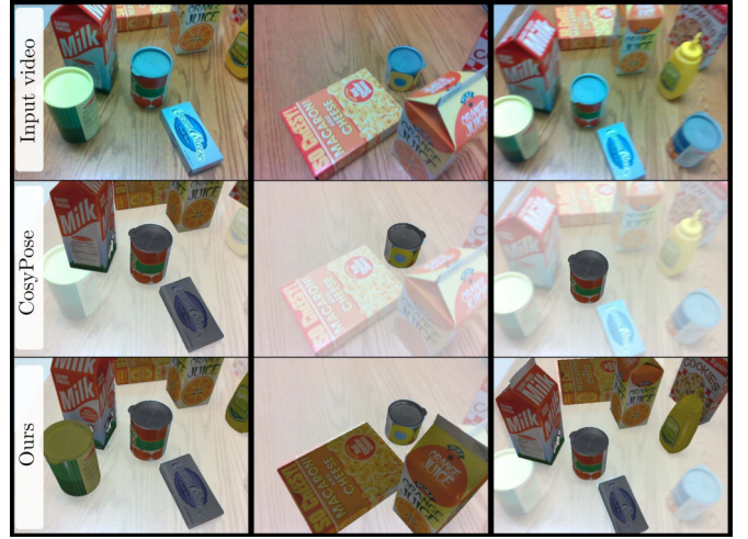
Fig. 4: Qualitative results on HOPE-Video. Comparison between our method and CosyPose [2] on HOPE-Video sequence (the first row). It can be seen that some of the objects are not detected by CosyPose (the second row). Our temporally smoothed predictions are shown in the last row, largely mitigating the issue of missing detections.
