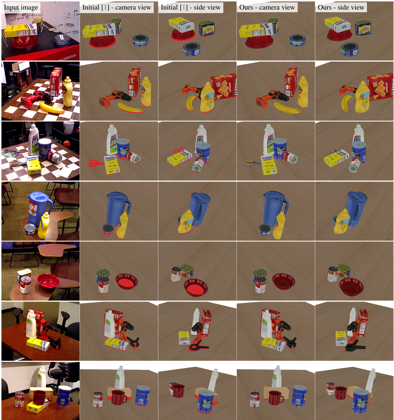
Figure 1. Qualitative results on the YCB-V dataset. We estimate initial object poses from an input image using MegaPose [1]. The resulting scene, shown from camera and side views, exhibits significant physical inconsistencies, with colliding parts highlighted in red. Our physical consistency optimization method significantly reduces these collisions, leading to a more plausible scene arrangement. Notice how our method successfully resolves collisions in the first two rows even though the objects are placed on top of each other.
