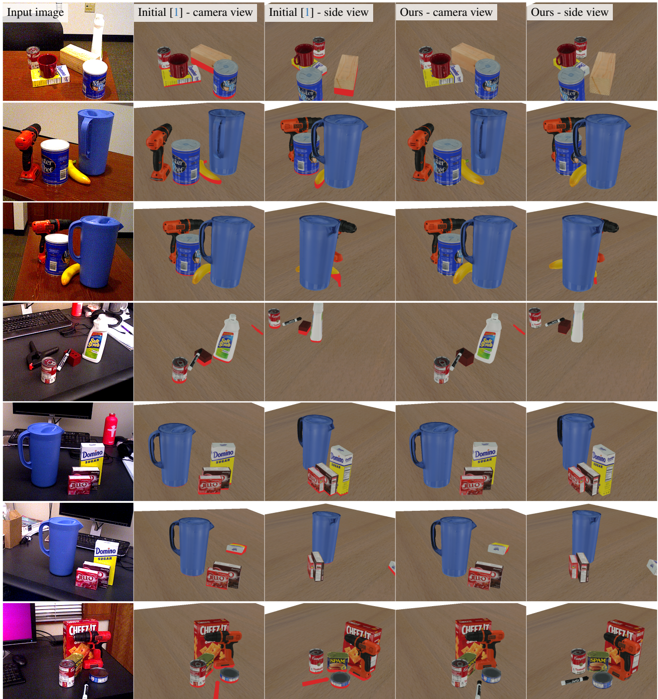
Figure 2. Qualitative results on the YCB-V dataset. We estimate initial object poses from an input image using MegaPose [1]. The resulting scene, shown from camera and side views, exhibits significant physical inconsistencies, with colliding parts highlighted in red. Our physical consistency optimization method significantly reduces these collisions, leading to a more plausible scene arrangement. Notice how our method successfully resolves collisions in the first two rows even though the objects are placed on top of each other.
